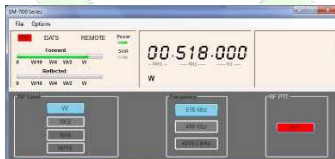
Navtex Operation Manager - INVELCO Navtex Transmitter Remote Control Screen
