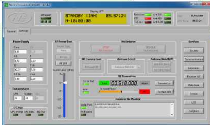
Navtex Remote Control - INVELCO Transmitter Control Screen.
