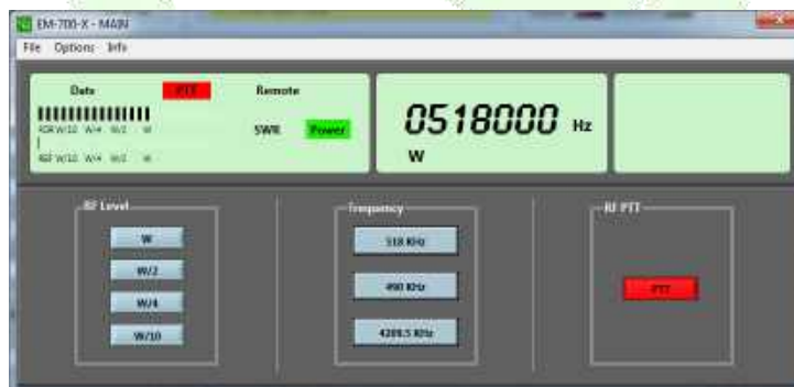
Navtex Remote Control - INVELCO Transmitter Control Screen.
